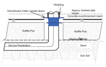
Ensure the HomeGuard<sup>®</sup> Collar being used is the correct size to suit the application e.g. 100 mm pipe requires a 100 mm HomeGuard<sup>®</sup> Collar – if the pipe is an un-common size you are required to create a sheet collar from either HomeGuard<sup>®</sup> TMB, PB, or DPC to achieve a tight snug fit – refer to the HomeGuard<sup>®</sup> Manual for instructions.
