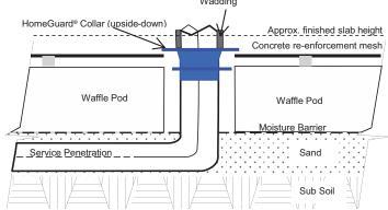
Ensure the HomeGuard® Collar being used is the correct size to suit the application e.g. 100 mm pipe requires a 100 mm HomeGuard® Collar – if the pipe is an un-common size you are required to create a sheet collar from either HomeGuard® TMB, PB, or DPC to achieve a tight snug fit.
