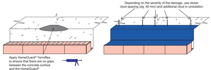
Note: Termiflex is a sheet bonding agent not a gap sealer, if slab is not indicative of the images above and damaged deeper than 6 mm contact contractor to repair.
